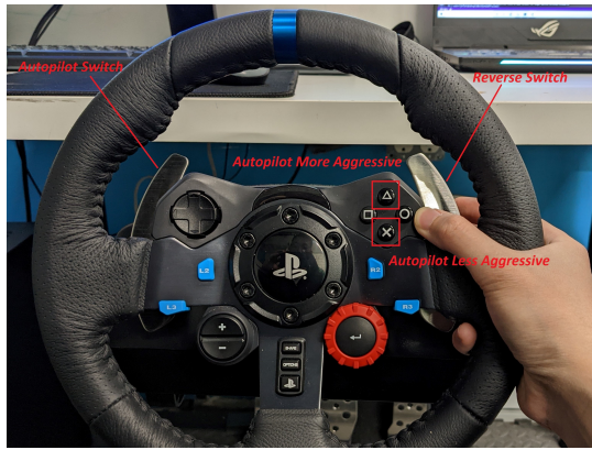
Fig. 4. Logitech steering wheel functionality explanation.
