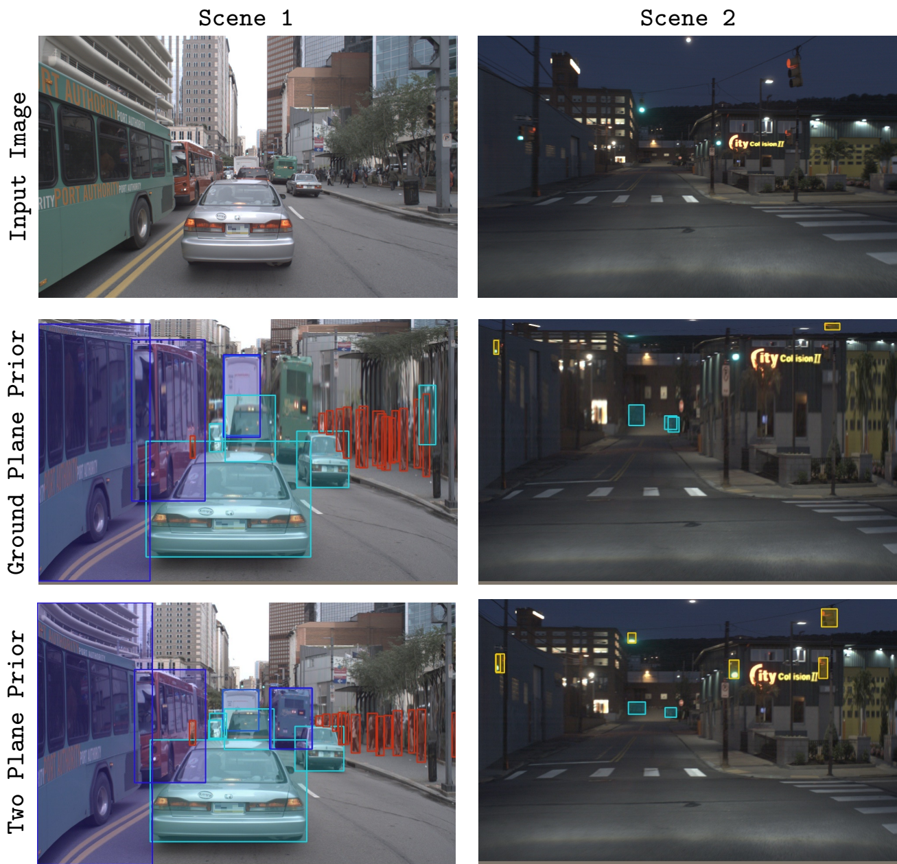
Figure 11. Ground Plane Prior vs Two-Plane Prior: This figure demonstrates how crucial it is to model the second plane. Learning is difficult with Ground Plane Prior (Section 5.1 in the manuscript) and causes heavy distortion of non-ground-plane regions.
