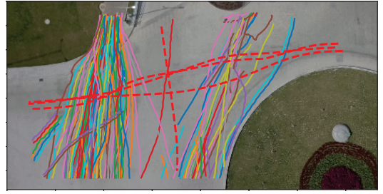
Fig. 6. Trajectories of vehicles (red dashed line) and pedestrians (colorful solid lines) in a clip of the shared space scenario.
