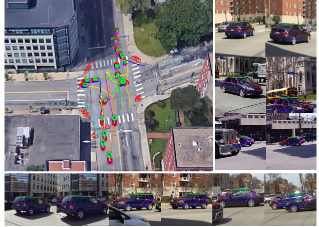
Figure 1: Reconstruction of vehicles crossing a busy intersection, making turns, going straight and changing lanes. A subset of vehicle skeletons (3D detector locations) and their 3D trajectories are augmented within the Google Earth view of the intersection. The reconstructions are reprojected into multiple views of two cars (a sedan and an SUV) demonstrating good performance under partial occlusions.
