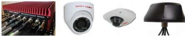
Fig. 2: Pictures of the Hardware. (From left to right: bus computer; exterior camera; interior camera; GPS and network antenna.)
