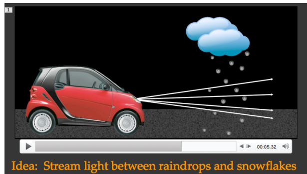
Figure 7: Driving in a snowstorm or rainstorm at night is incredibly hard. The snowflakes and raindrops are illuminated brightly and distract the driver from observing the entire road. The smart headlight has unprecedented resolution over angle and time so that beams of light may be sent in between the falling rain and snow.
