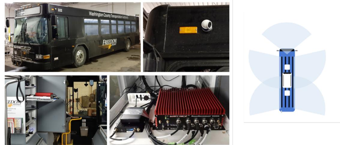
Figure 5.1: The left four images show the commuter bus, an image of the computer, the cabinet that contains the computer and electronics, and one of the cameras. The right diagram shows the field of view of each installed camera, where one faces forward and four side cameras face opposite directions from each other.
