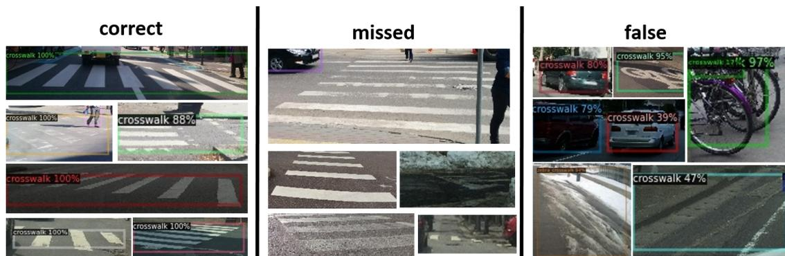
Figure 4.5: Qualitative results from crosswalk predictions: CARLA-trained model tested on MVD dataset. Shown are correct, missed and false detections.
