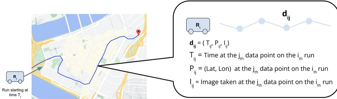
Figure 3.3: Illustration of the data points collected along the  $i_{th}$  run of the bus
