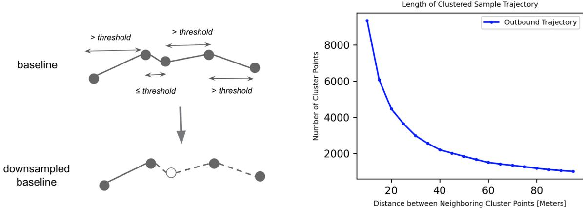
Figure 3.7: (Left) The dense baseline trajectory is downsampled based on a distance threshold to neighboring points. (Right) The number of points on the baseline trajectory decreases exponentially as we increase the distance threshold.
