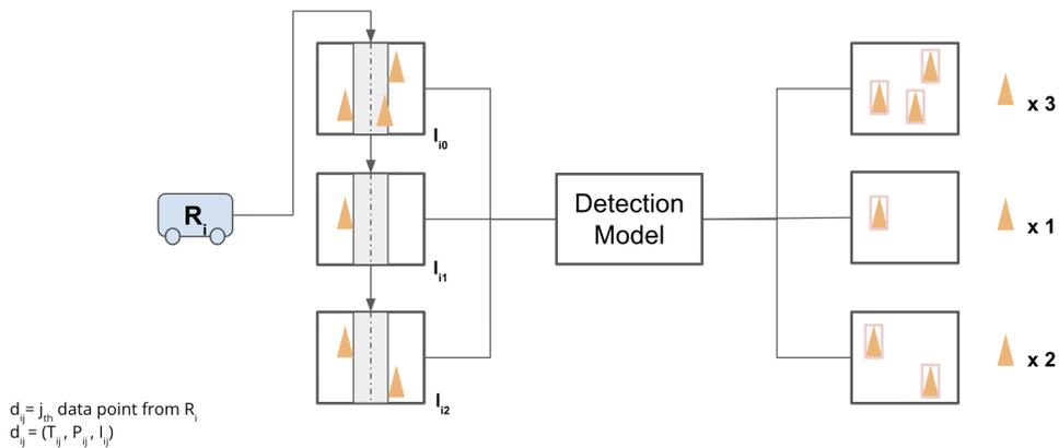
Figure 4.1: For each data point on a run, we assign an anomaly score that indicates the likelihood of that scene being a work zone.
