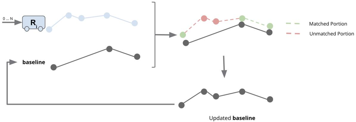
Figure 3.6: The collection of bus runs are iteratively clustered into a dense baseline trajectory.
