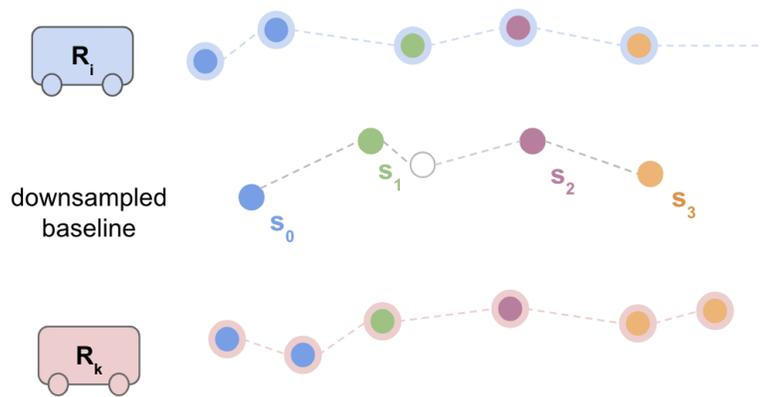
Figure 3.8: Data points on each run is assigned to its nearest point on the downsampled baseline trajectory.
