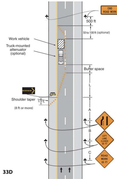
Figure 2.3: An illustration of a short-term stationary setup. The distances A, B, C should be proportional to the work zone speed limit. TTC Signs are placed some distance prior to the actual work zone. Delimiters are placed surrounding the boundaries of the work zone. [2]
