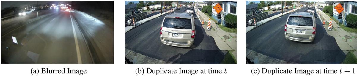
Figure 3.4: (a) Images taken before sunrise tends to result in high-blur images. (b) and (c) is a pair of consecutive frames that are taken when the vehicle is stationary. This will generate a pair of images that are close duplicates of one another.
