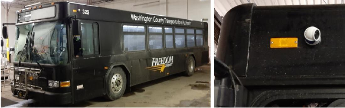
Figure 3.2: Pictures of the Transit Bus and its Exterior Cameras [32]
