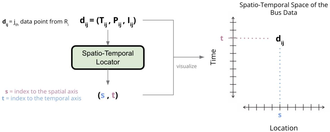
Figure 3.5: Overview of the alignment process: for each data point  $d_{ij}$ , we map it to a location on the discretized 2D space formed by a spatial and temporal axis.
