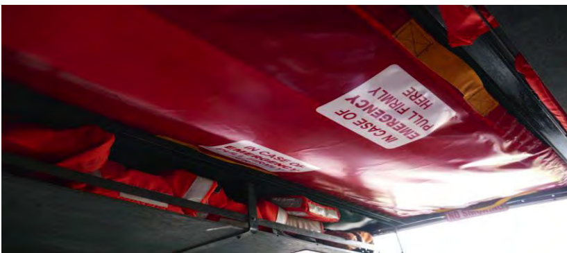
FIGURE 5-10 Pull open canopy section, Original Wisconsin Dells. SOURCE: T. Graul, committee member.
