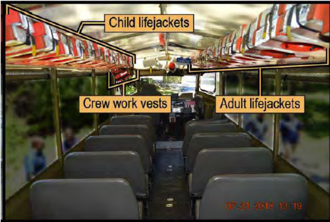
FIGURE 5-1 Stowage of life jackets under the canopy from Stretch Duck 7 .
