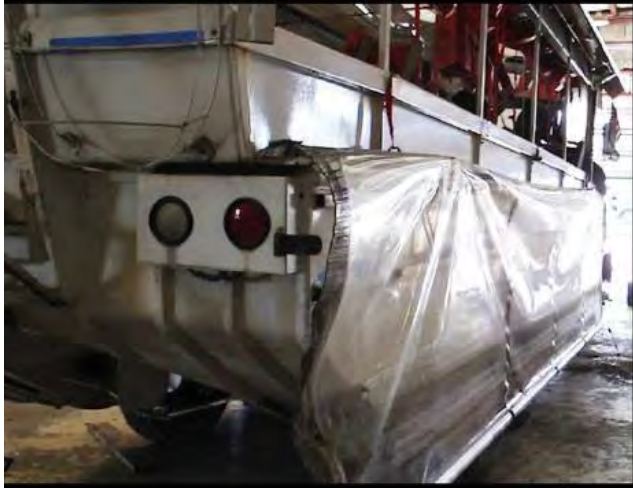
FIGURE 5-4 Side curtain released for emergency exit.
