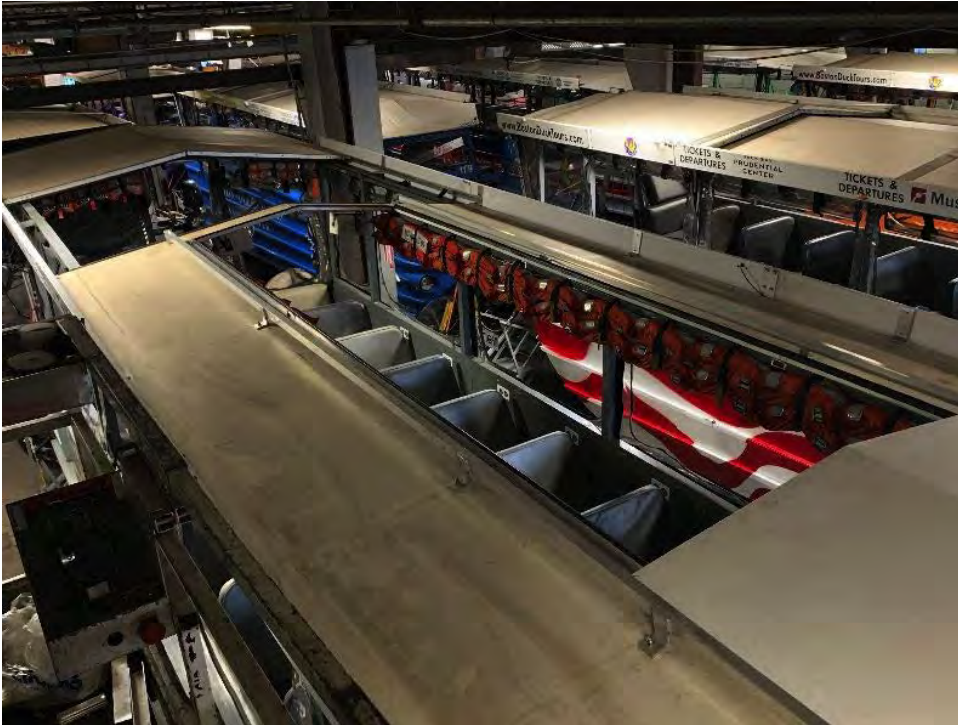
FIGURE 5-9 Slide roof panels with centerline hatch, Boston Duck Tours. SOURCE: T. Cerulle, Boston Duck Tours.
