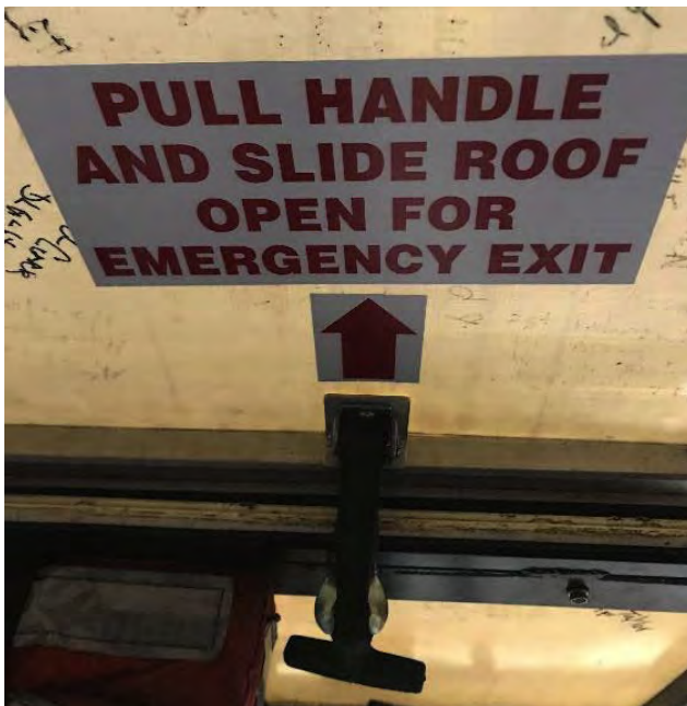
FIGURE 5-8 Emergency handle with manual pull for sliding roof, Boston Duck Tours.
