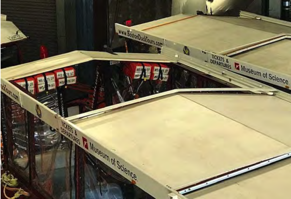
FIGURE 5-7 Stern area slide roof on Boston Duck Tours.
