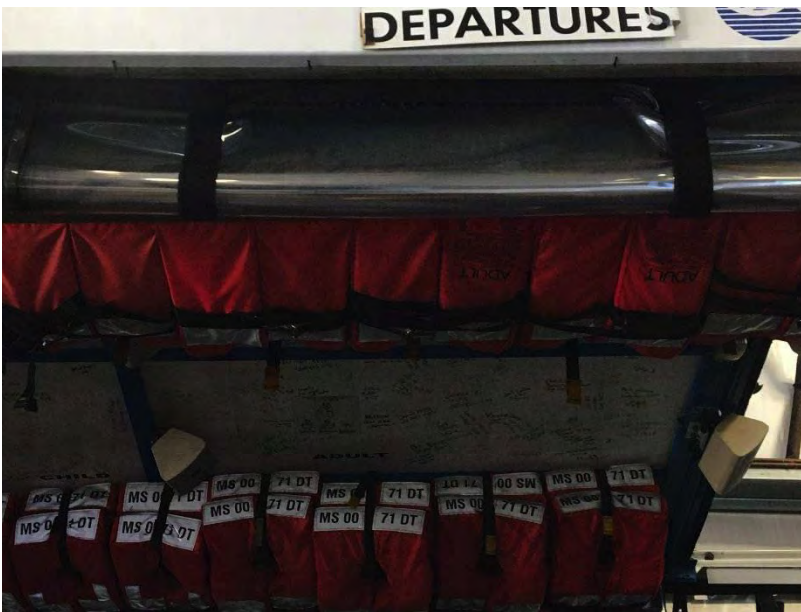
FIGURE 5-13 Side curtain in rolled up position, Boston Duck Tours. SOURCE: R. Cook, committee member.
