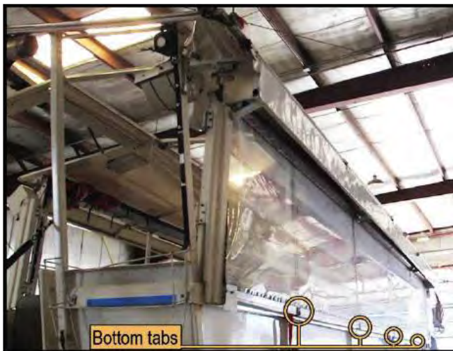
FIGURE 5-3 Side curtain rolled down to protect passengers.
