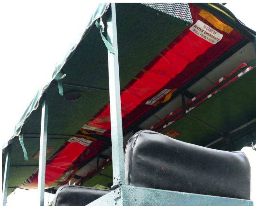
FIGURE 5-11 Pull down canopy section on length of centerline, Original Wisconsin Dells. SOURCE: T. Graul, committee member.
