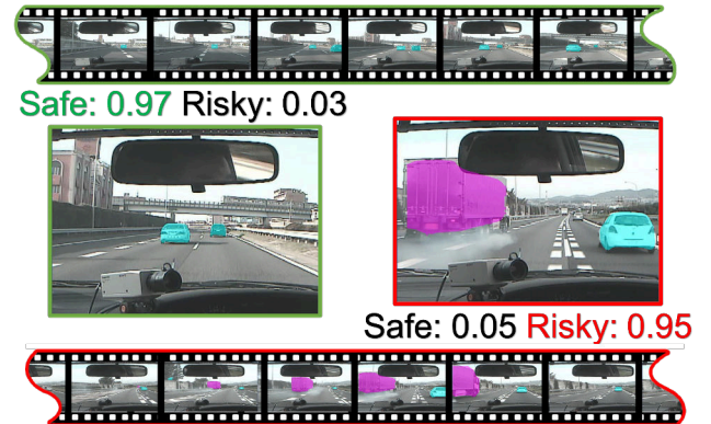
Fig. 1. Two lane change samples and classification outputs of our method. The average duration of these clips is \sim 10 seconds. 0.937 AUC score was achieved with the proposed method. Video samples can be found in our repository 1 .
