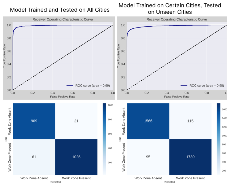
Figure 19: Detection model performance as illustrated by the receiver operating characteristic curve and confusion matrix. The results on the left column are for the scenario where images from all cities form the training and testing data sets, while the right column has cities split into training and testing.
