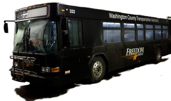
Figure 3.2: A bus similar to the one in this images has been equipped with cameras, sensors, and a mobile computer to capture the data used in this implementation. Source: Rotondo et al. [89].
