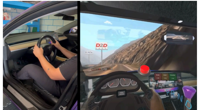
Figure 1. Mixed Reality Driving. Sensors affixed to the steering wheel and pedals of the vehicle allow the driver to use his real vehicle (on the left) to drive the Google Earth Environment (right).
