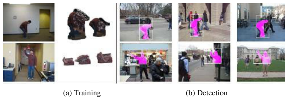
Figure 1. Example of video processing in which reference actions (shown in (a) in prototypical videos) are recognized in input videos (example frames in which the action is detected are shown in (b)).
