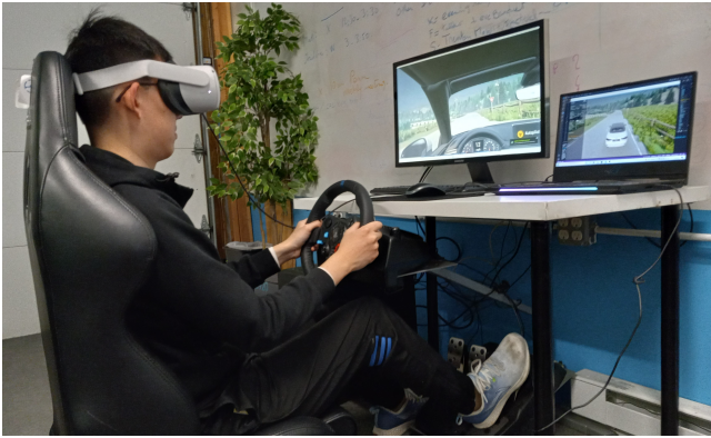
Figure 2: Simulator demonstration: left monitor shows CARLA server first person driver’s view which is also displayed in the VR headset; right monitor shows the CARLA client third-person tracking view which is provided by the CARLA client by default.
