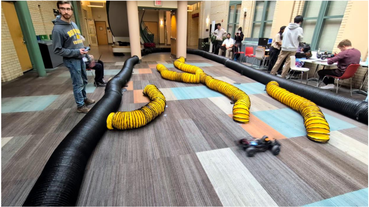
Figure 3. Track set-up and single car participating in Race 2 in the Spring 2026 offering of the CMU F1Tenth Autonomous Racing course. Whereas Race 1 required only reactive maneuvering, Race 2 required mapping and localization.
