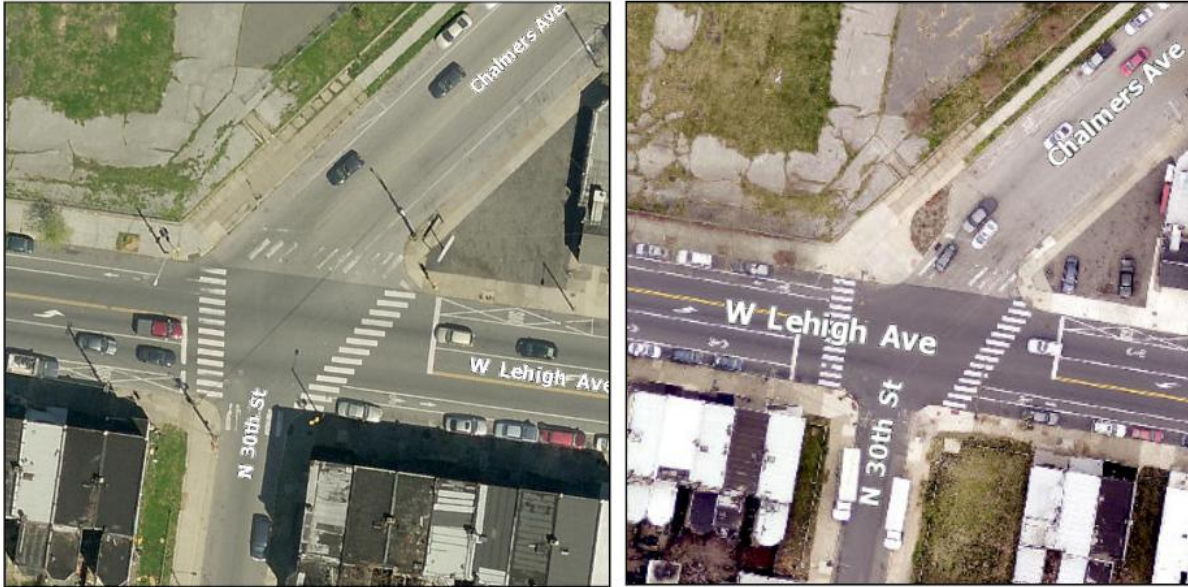
Figure 2: Before and after imagery of curb extension at NW corner of Lehigh Ave, Chalmers Ave, and 30th St in North Philadelphia
