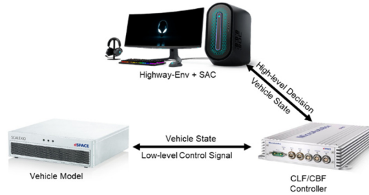
Figure 4.17. HIL setup for evaluating the proposed hierarchical control framework [115].
