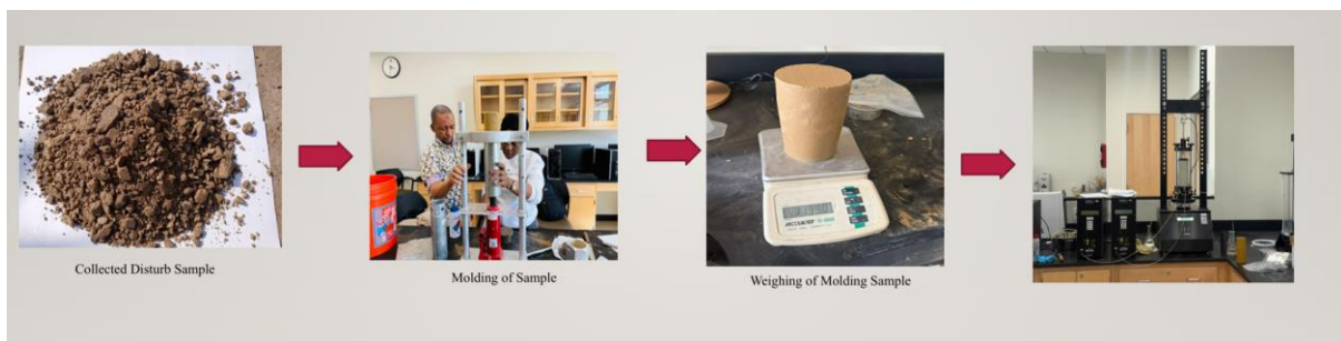
Figure 3.4: Sampling and preparation for CU triaxial Test.
