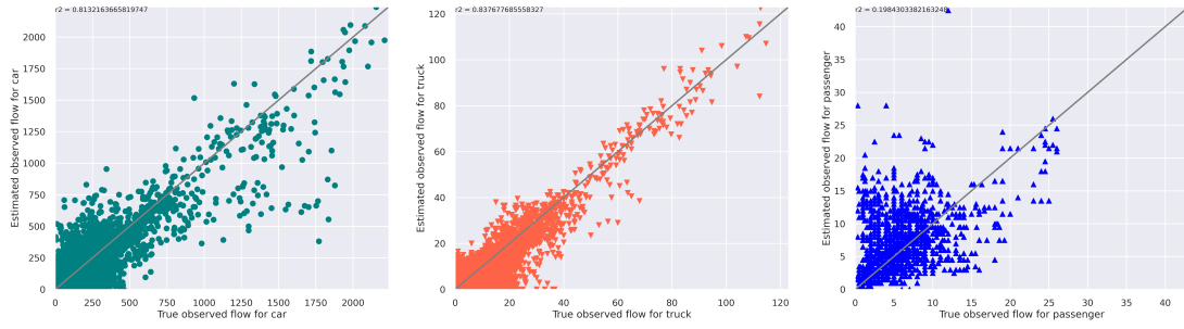
Figure 12: Estimated and true observed flow for cars, trucks, and passengers for the network in the central Ohio region (unit: number of vehicles / 15 minutes or number of passengers / 15 minutes)
