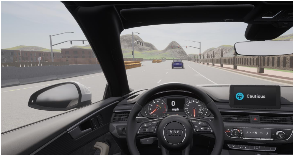
Fig. 11. Highway scenario in the first-person driver's seat view. Current autonomous driving mode is set to cautious, other available options: normal, aggressive.
