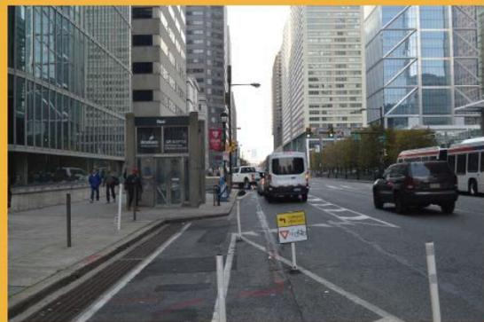
**Figure 2. Study Segment.** a, The study corridor. Road segments are either characterized as protected by bollards, which are flexible and collapsible delineators that line the bicycle lane spaced approximately 1.5 meters apart, or being conflict zones (highlighted in yellow), where bicycles and vehicles mix, and bicycles are not protected. b, sample infrastructure map with conflict zones highlighted. c, Sample photographs of protected and unprotected segment cross-sections.
