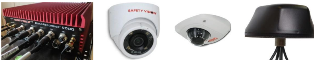
Figure 7: Some pictures of the hardware on the bus. From left to right: bus edge computer; exterior camera; interior camera; GPS and network antenna.
