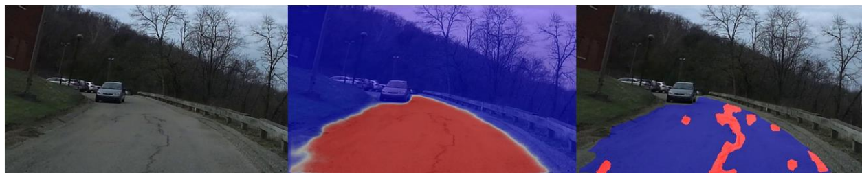
Figure 2: Left: Raw image. Middle: Detection of road area. Right: Detection of cracks.
