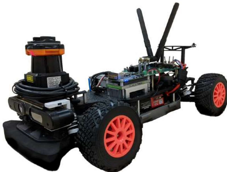
Figure 1. F1Tenth Autonomous Vehicle
