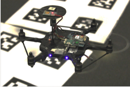
Fig. 13. Autonomous hexrotor with downward-facing camera flying over synthetic features.
