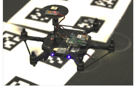
Fig. 3. Autonomous hexacopter with downward-facing camera flying over synthetic features.
