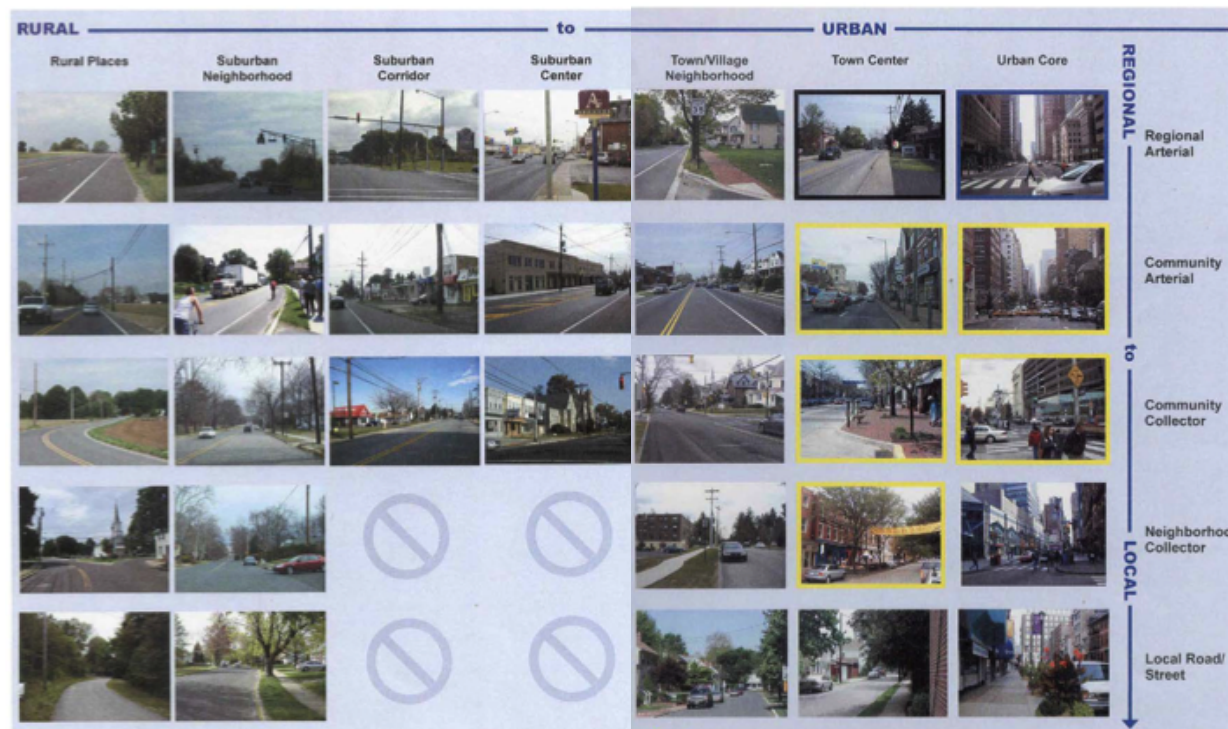
Figure 5 | The 2010/2015 Design Manual's Figure 1.2 Illustrated Roadway Typologies also includes suburban roadway settings that bridge between the earlier urban and rural locations, without changing the basic topological framework. This matrix is a useful tool for transportation planners in understanding how context and scale create identifiable, and differentiated, characteristics.
