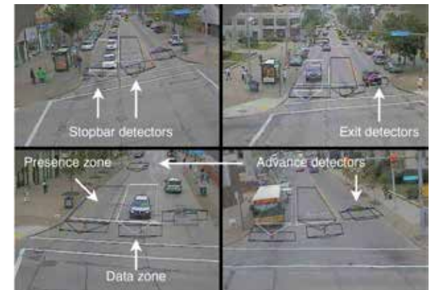
Figure 46 | The placement of detectors in a typical installation of SURTRAC's adaptive signalization.
