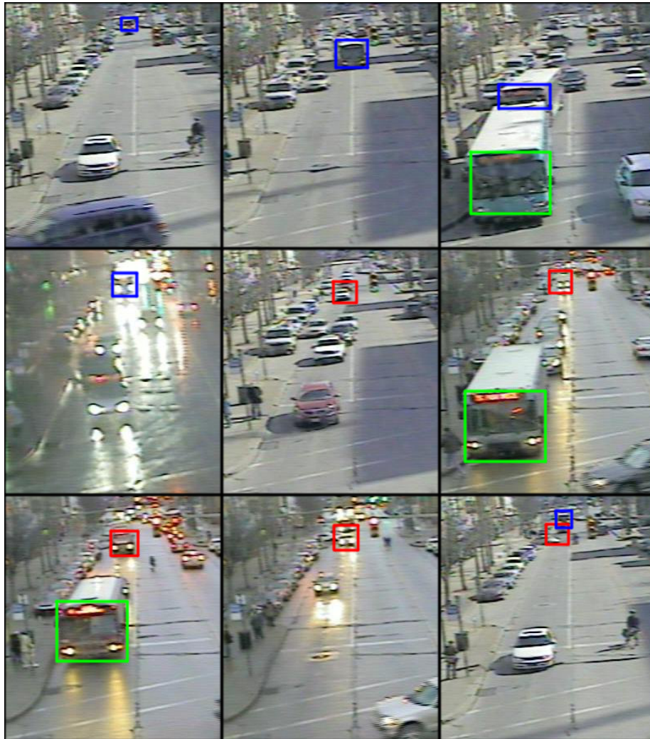
Figure 11: Bad detections by our system with threshold 0.98. It misses buses more often in difficult situations (top row and middle left - blue boxes). False positives occur with certain car configurations and occasionally with trucks (bottom row, middle middle and middle right - red boxes).
