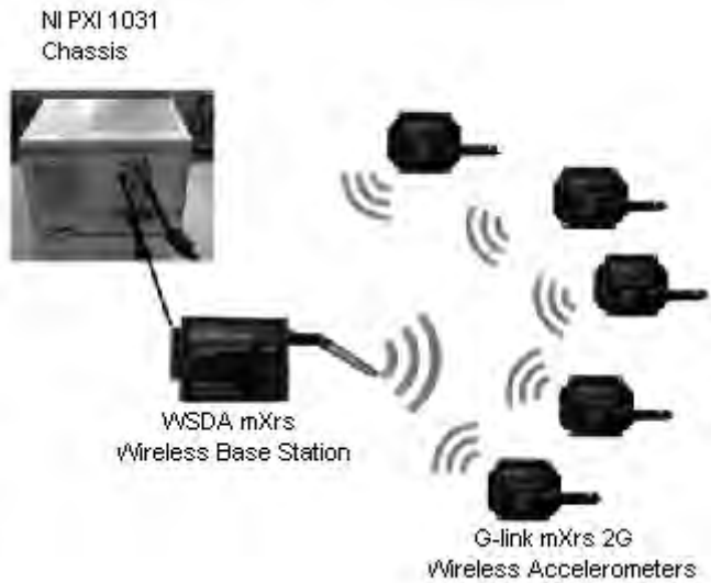
Figure 5. Data acquisition equipment
