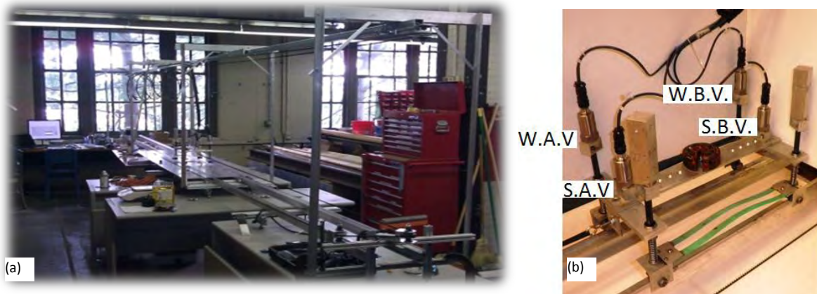
Figure 16: Experimental setup. a) General angle photo of experimental setup, b) Vehicle picture. W.A.V. is the wheel level on the A axle, and S.A.V. is the suspension level on the A axle. W.B.V. and S.B.V. are the corresponding wheel and suspension levels on the B axle.
