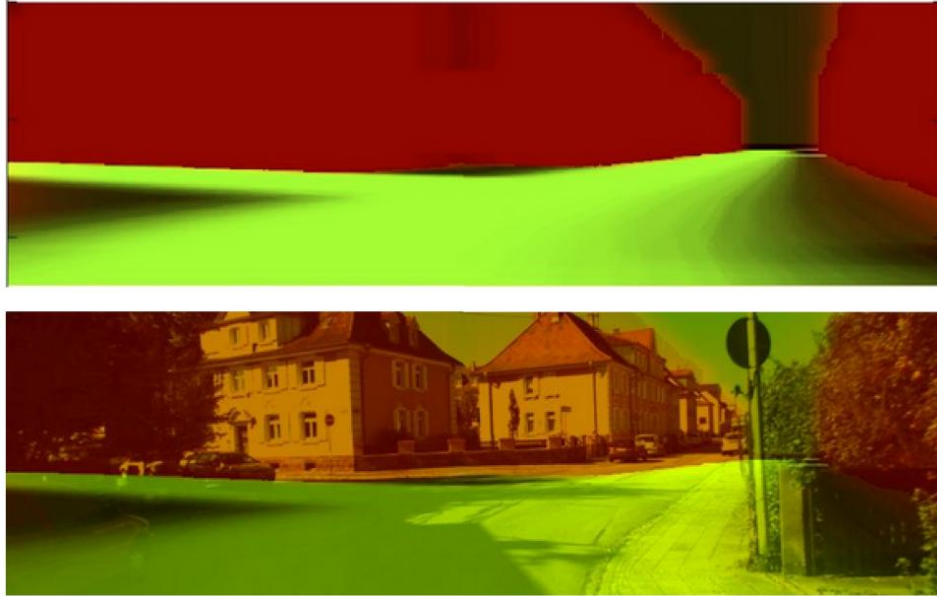
Figure 3. Map prior with position uncertainty (top); original image overlaid with prior (bottom). Buildings are indicated in red, and the roads in green. A higher color saturation indicates higher certainty, while lower saturation indicates higher uncertainty.
