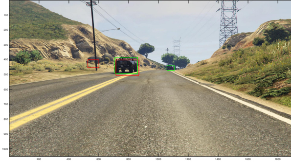
Fig. 3. GTA frame with red bounding boxes around cars detected by YOLO, and green boxes around true cars. Note the red box around the bush on the left, indicating a YOLO false positive, and the lack of red box around the faraway car on the right, indicating a YOLO false negative. The red box in the middle is a true positive.
