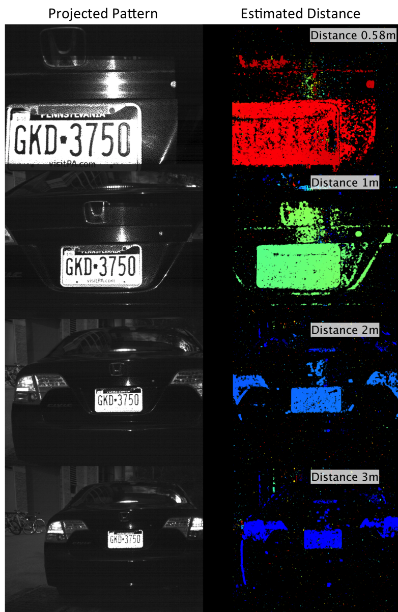
Figure 6: The patterns projected by the system are shown on the left side. Example distance maps to a vehicle's license plate are shown on the right.
