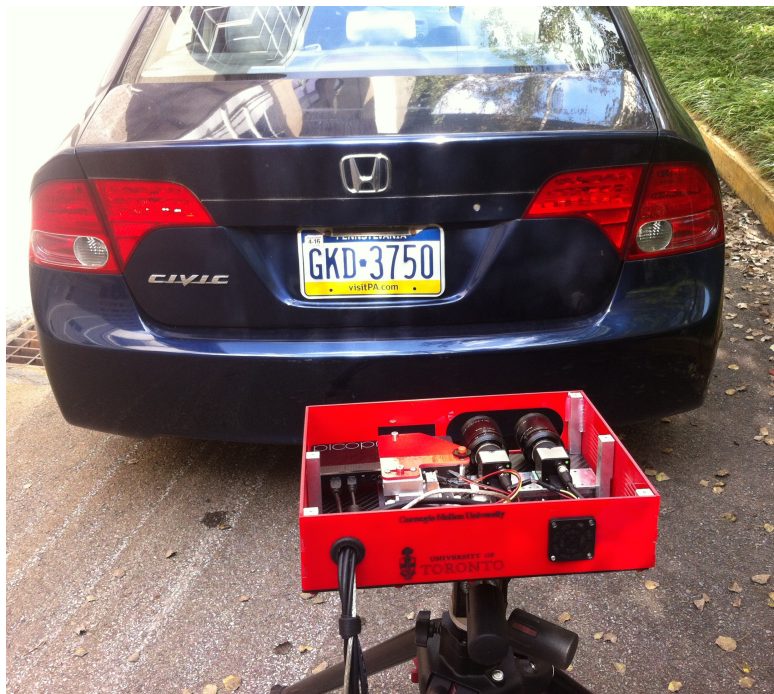
Figure 5: The position of the system relative to a vehicle during an experimental run. The vehicle was in direct sunlight and 0.5 to 3 meters in front of the system.
