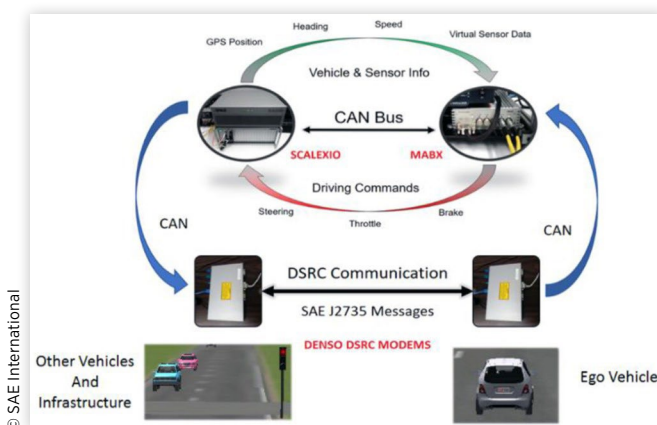
FIGURE 14 HiL equipment and communication.
