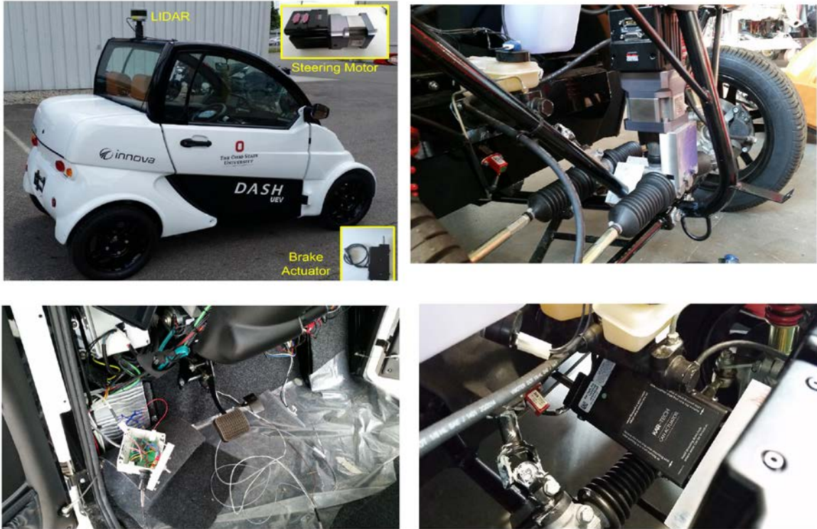
Figure 3. Dash EV drive-by-wire system.
