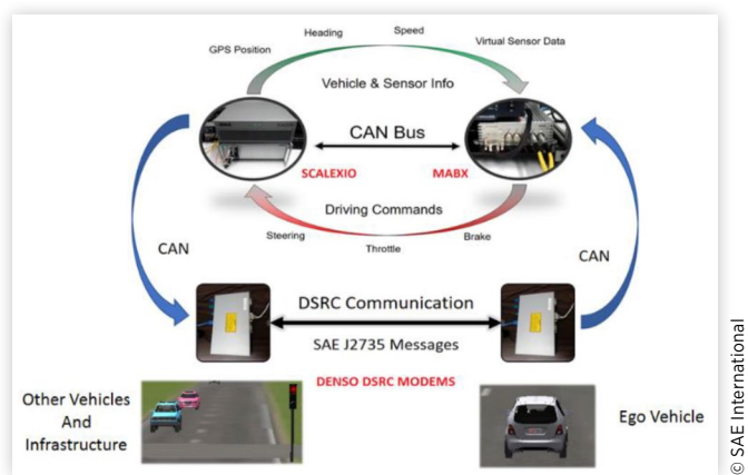
FIGURE 15 HiL equipment and communication.
