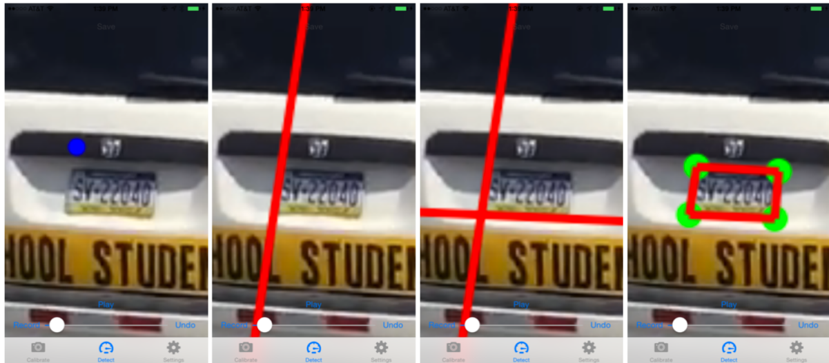
(a) User selects one point along an edge (b) User selects another point, completing the edge (c) User repeats the process for the next edge (d) After four edges are specified, the corners are found
