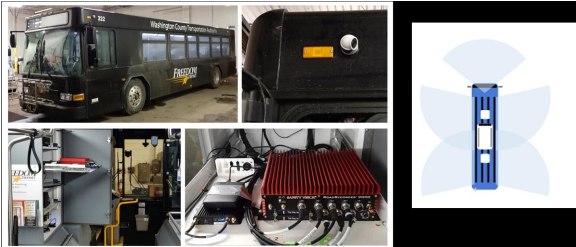
Figure 1 The left four images show the commuter bus, an image of the computer, the cabinet that contains the computer and electronics, and one of the cameras. The right diagram shows the field of view of each installed camera, where one faces forward and four side cameras face opposite directions from each other.
