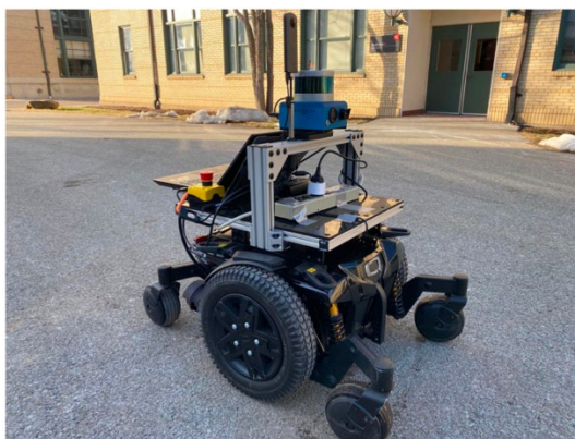
Figure 10: The wheelchair robot platform used in our experiments is equipped with a 4.1 GHz i7 computer and a NVIDIA GTX 1660Ti GPU card.
