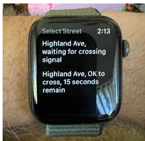
Figure 6: An initial wearable version of PedPal+
