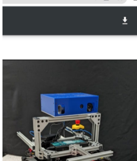
Figure 13: Full-stack autonomous wheelchair with Programmable Light Curtain sensor attached.
