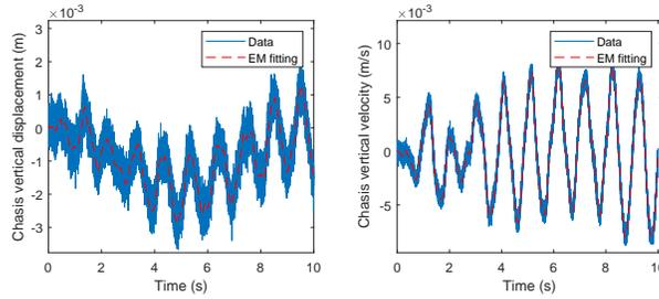
Figure 2. Simulated vertical displacement and velocity of the moving vehicle (blue curves) and the fitting results of them by the EM-algorithm (red curves).
