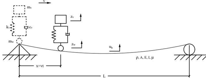
Figure 1. Model of a two-degree of freedom oscillator moving over a single-span, simply supported beam with a constant velocity.
