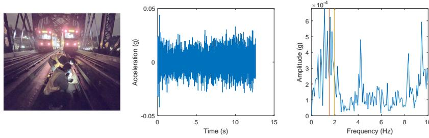
Figure 3. Picture of the experiment and an acceleration record collected from the vehicle while was passing over the bridge. The second subplot shows the raw acceleration signal, and the third subplot presents the amplitude spectrum of the acceleration. The vertical line in red and yellow indicate the natural frequency of the vehicle and the bridge, respectively.
