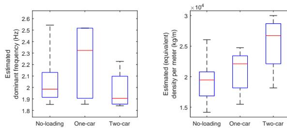
Figure 4. Evaluation results of our proposed approach. The first and the second subplots show boxplots of the estimated dominant frequency and unit length density of the bridge. The red dashed line indicates the natural frequency of the bridge estimated by free vibration tests.
