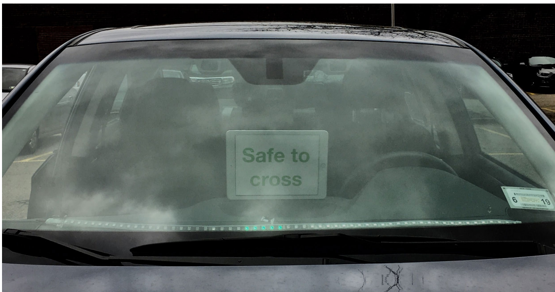
Figure 2. Pedestrian crossing, LEDs indicate AV is tracking the pedestrian's motion
