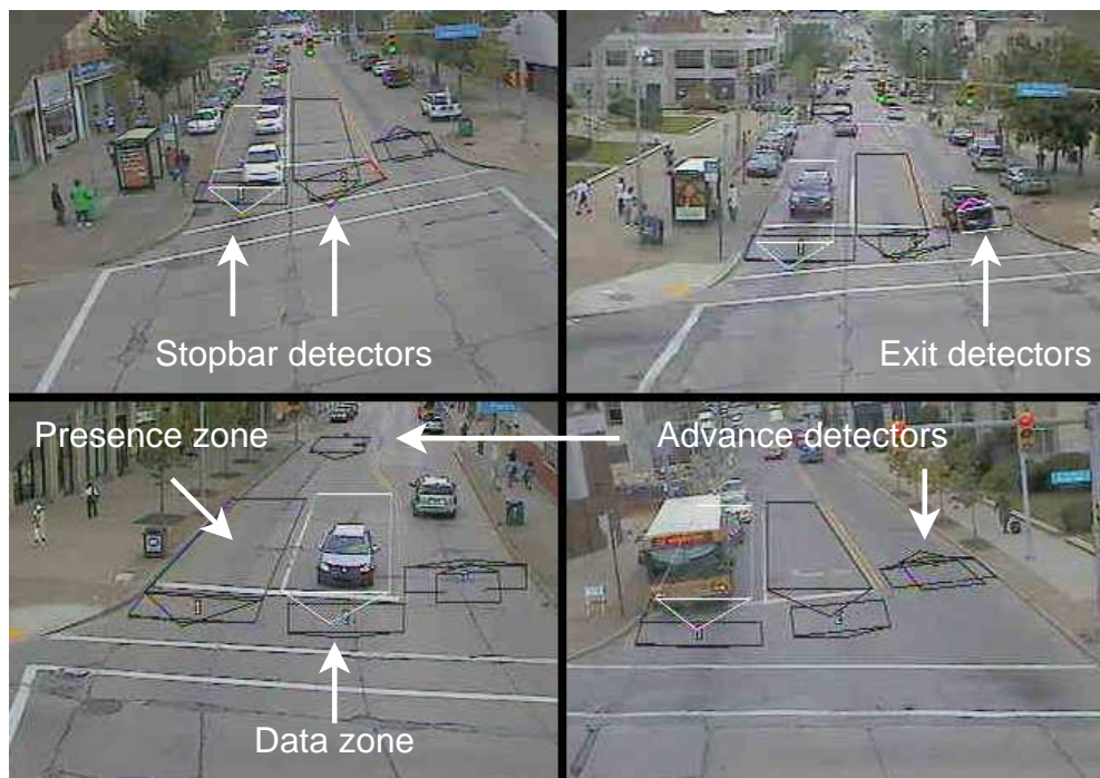
FIGURE 2 The placement of detectors in a typical installation.
