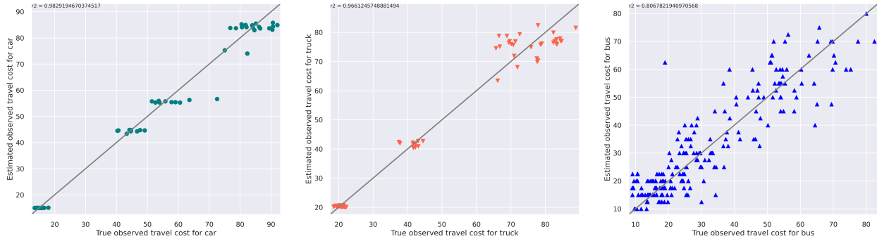
FIGURE 8 Estimated and “true” observed cost for cars, trucks, and passengers for the small grid network (unit: second)
