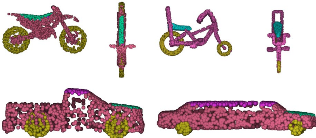
Figure 6 Successful segmentation of point clouds. The motorcycle and bicycle are segmented into frame, saddle, and tire, the cars are segmented into wheels, roof, hood and body.
