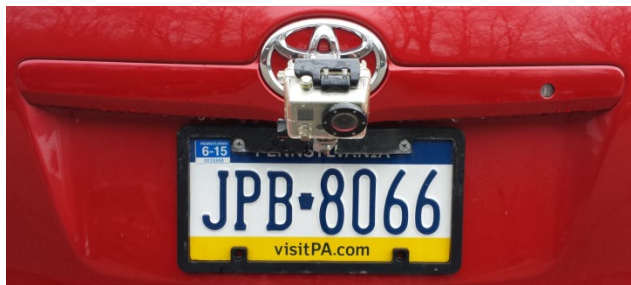
Figure 1: Data Collection Set-up
