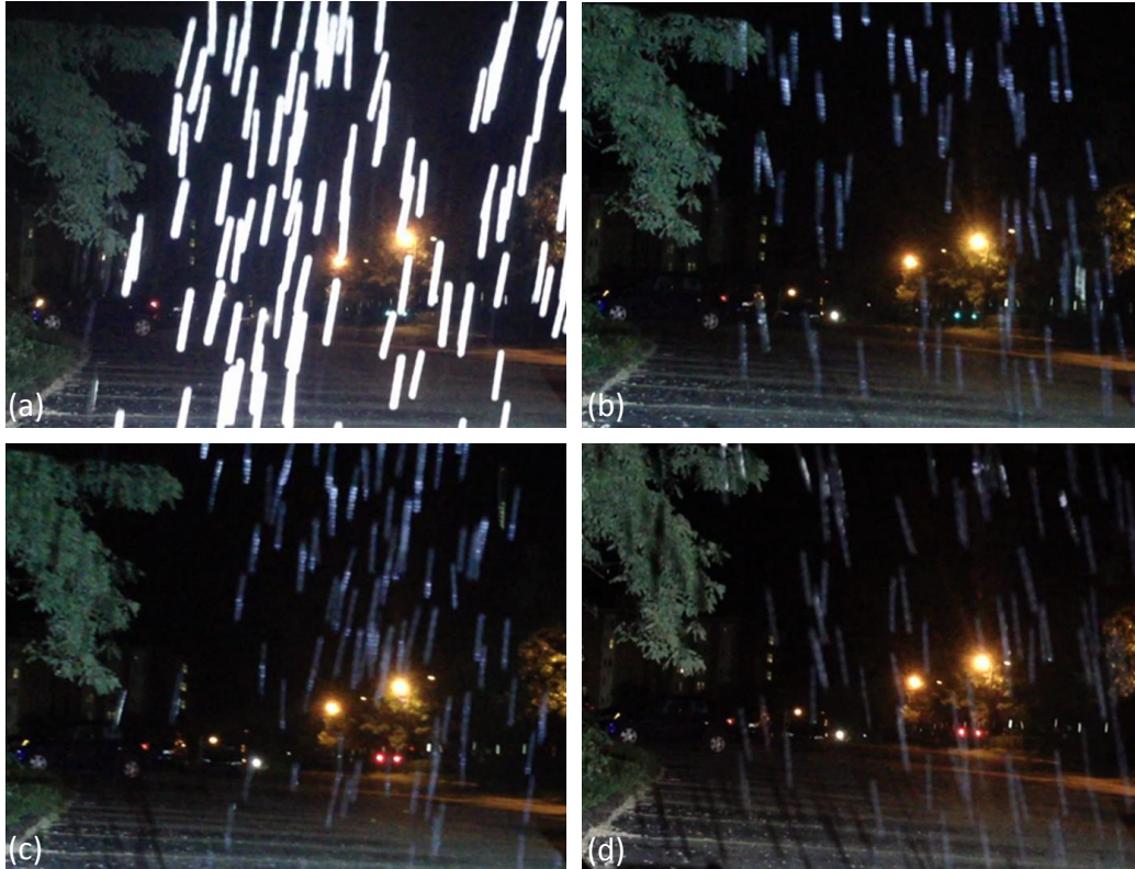
Figure 5.15: Visual evaluation of system performance for small objects moving chaotically. Artificial snowflakes are dropped. Still frames from a video captured at 30 fps are shown. In (a), snowflakes are constantly illuminated. In (b)-(d), snowflakes are adaptively dis-illuminated while increasing the size of the dilation kernel resulting in higher system accuracy and lower snowflake visibility.
