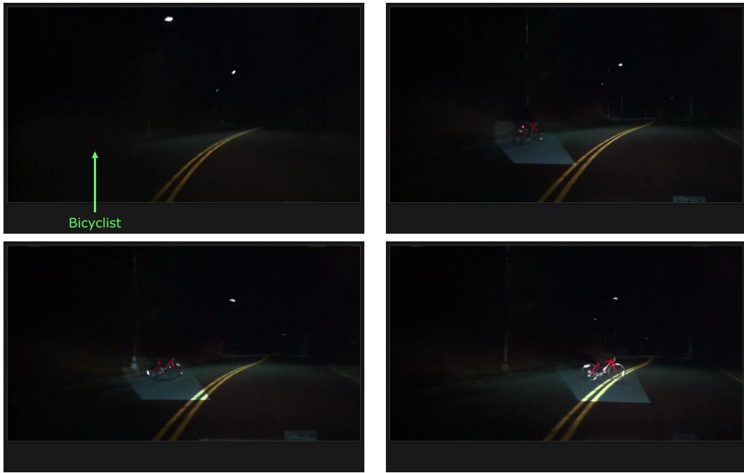
Figure 6.7: Example of spotlighting a bicyclist to provide an early visual warning for driver's on the road. In the first image, the bicyclist is difficult to see even with the high beams on. In subsequent images, the bicyclist crosses the road as our headlight detects it and illuminates the road in the direction of the bicyclist and the bicycle itself. The bicyclist is intentionally not spotlighted to avoid glaring him.
