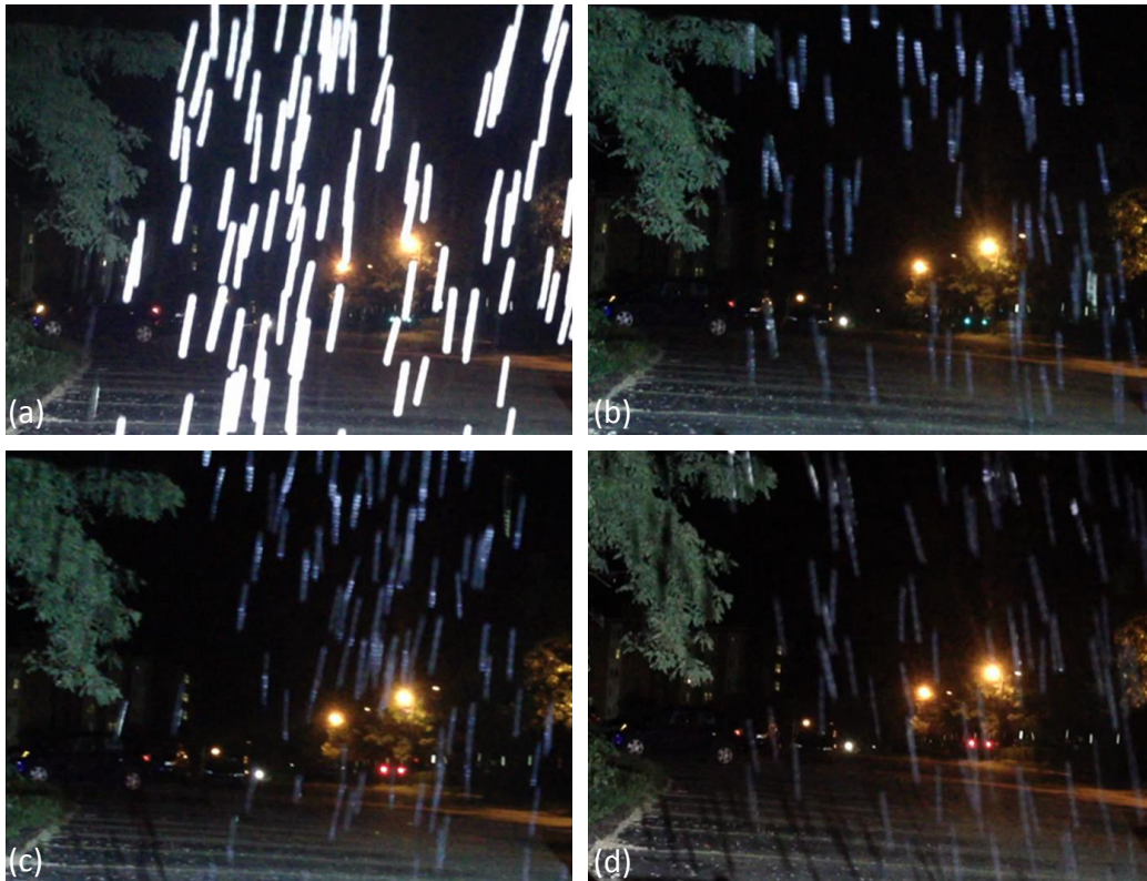
Figure 6.5: Visual evaluation of system performance for small objects moving chaotically. Artificial snowflakes are dropped. Still frames from a video captured at 30 fps are shown. In (a), snowflakes are constantly illuminated. In (b)-(d), snowflakes are adaptively dis-illuminated while increasing the size of the dilation kernel resulting in higher system accuracy and lower snowflake visibility.
