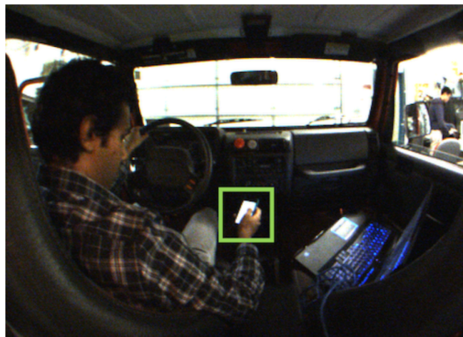
FIGURE 1. View from an over-the-shoulder camera of the interior of a vehicle. The vision-based approach developed in this project detects the use of a cell-phone by the driver of the vehicle (green box).
