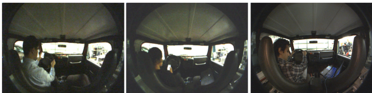
FIGURE 2. Images captured by the Pointgrey Flea2 camera mounted with a Fujinon Fish-eye lens. The three drivers have visually different driving styles and seat adjustment preferences. Additionally, while drivers 1 and 2 (from left) use the cell phone around the steering wheel, driver 3 only uses the phone at waist level.
