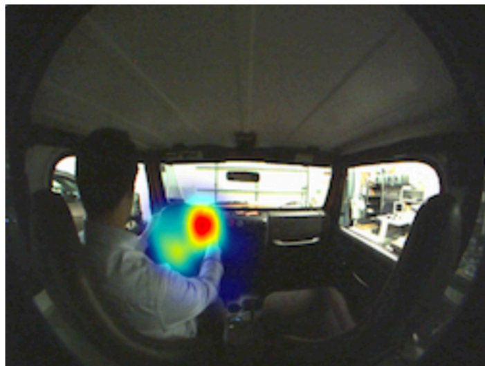
FIGURE 6. The mask within which the detection is performed is overlaid has a heatmap. The current driver is dominantly right-handed. Consequently, the heatmap is relatively focused to capture the region spanned by the driver's right hand.
