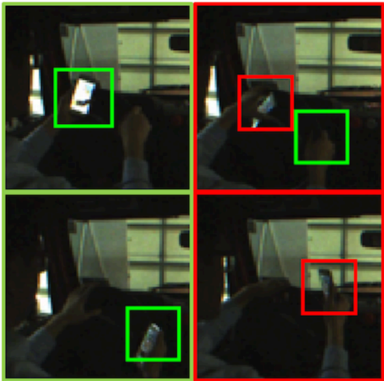
FIGURE 11. The images on the left show correct detections when the driver uses the phone with the left hand, and over the steering wheel. The failure cases are shown in the right column. The large appearance change caused by out of plane rotation causes the detection to fail.
