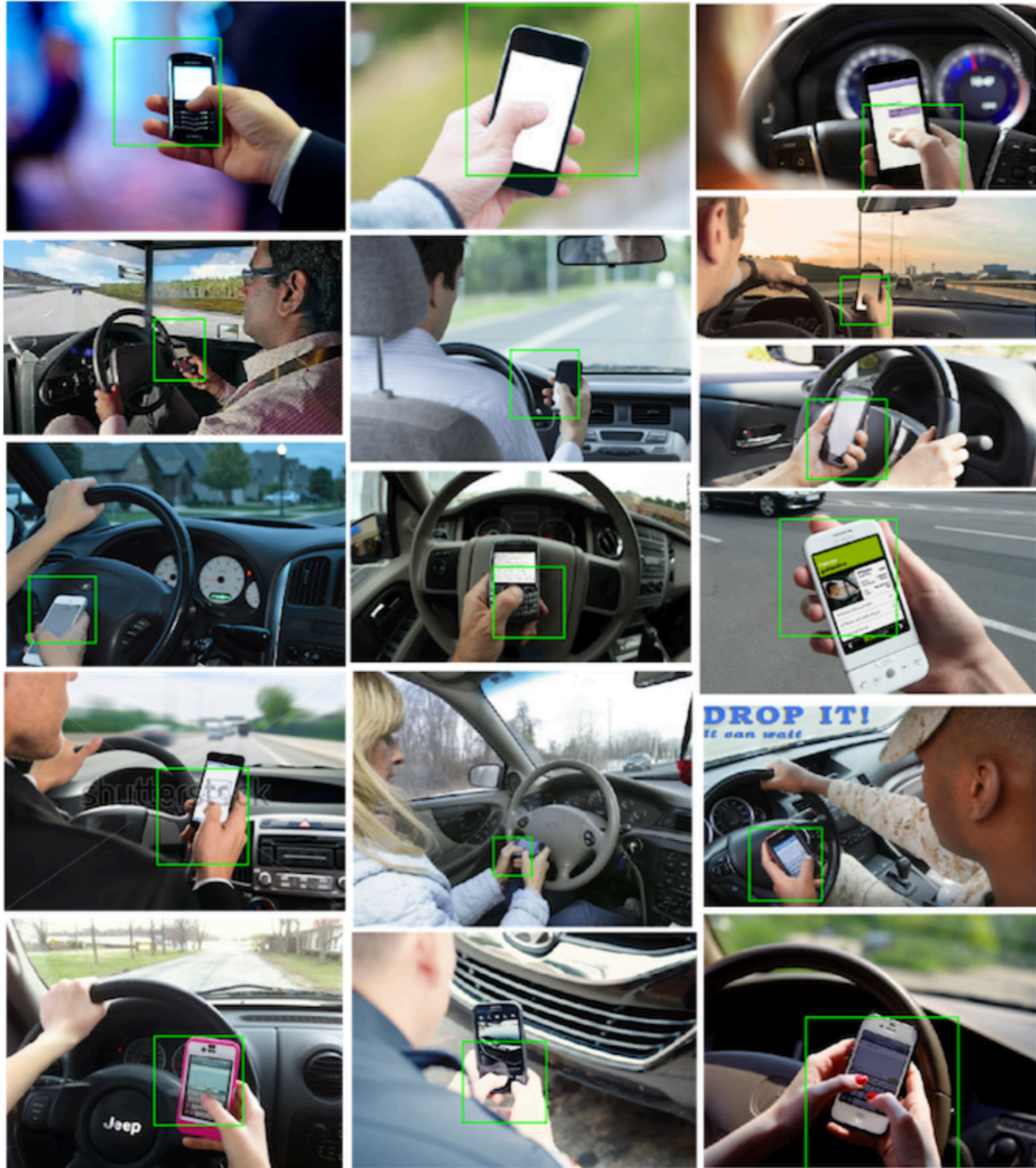
FIGURE 12. Successful detection results on test data. The figures on the left column show the driver switching hands for phone use. The location of the camera was slightly shifted for the figure on the right, and the light at the interior of the vehicle was switched-on resulting in different lighting conditions.
