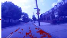
Classification using segmentation of ground [1], SLIC segmentation [2], bag-of-words, and support vector machines.
