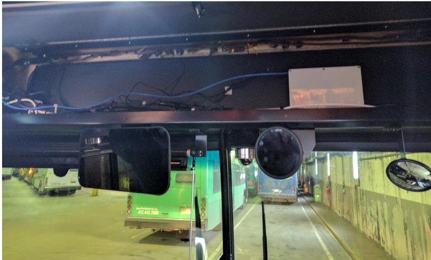
Figure 7: OBU Install location on shelf above the front window.
