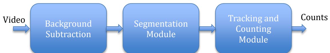
Figure 2: Block diagram of vehicle tracking architecture
