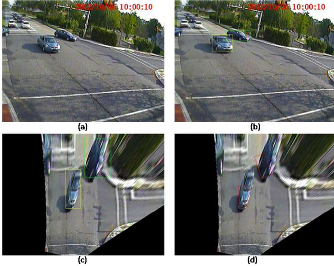
Figure 1: Sample frame (a) grouped in original perspective (b) and in "top view" perspective (c), and the size of the reconstructed vehicle represented by the red bounding box (d).
