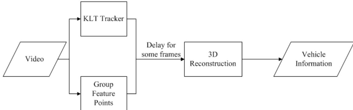
Figure 2: Block diagram of proposed approach.
