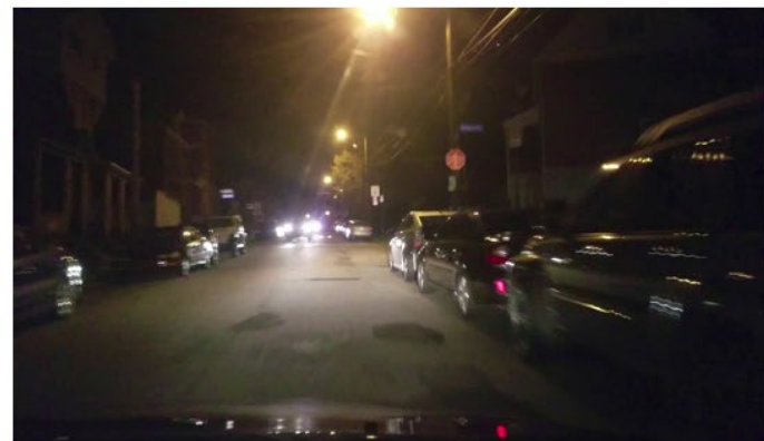
Figure 4 Retroreflectivity of the traffic sign are indicated by their brightness. On top right is a sign with good retroreflectivity. The intensity of the red channel is high, almost to the point of saturation (value around 255). On the bottom right is a faint stop sign. The intensity in the red channel is much lower, around 150.
