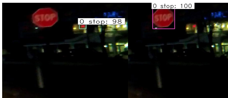
Figure 3 Stop sign detection at night. On the left is one failure case where a red light is mistaken for a stop sign. On the right is a correct detection.
