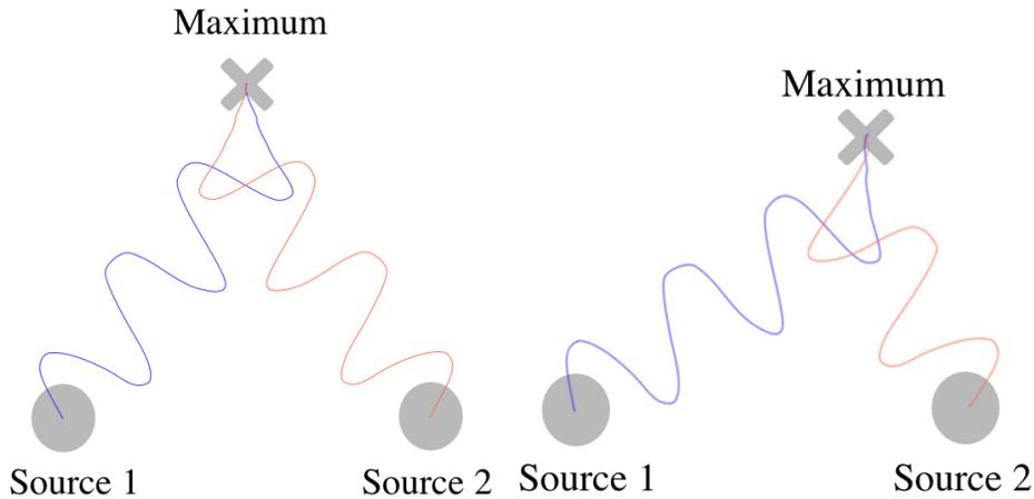
Figure 2: Position of maximum with uniform-phase sources and out-of-phase sources.
