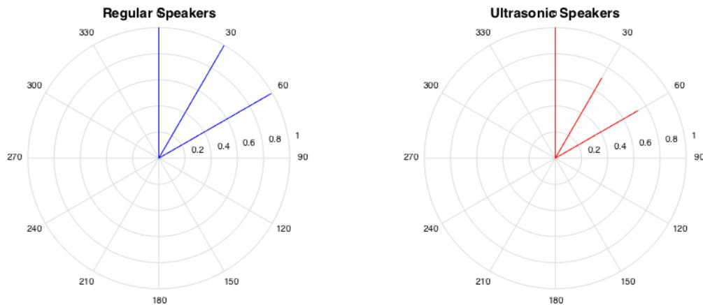
Figure 1: Comparison of relative signal strength at various angles for a regular speaker and an ultrasonic speaker
